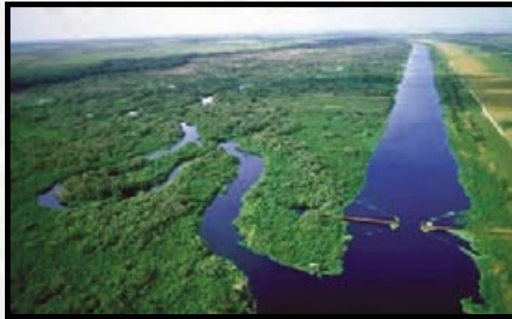
A South Florida Water Management District photo shows how the artificial river channel on the right short-circuited the original winding river.
