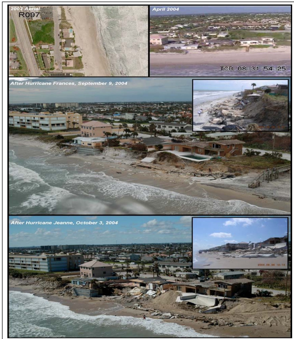
Shell Street - Scale of scour and dune erosion after Hurricanes Frances and Jeanne (R97), City of Satellite Beach
